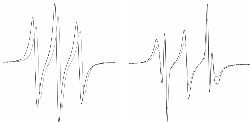
Figure 6.3 L-band ESR spectra of left) a HD-PMI (1 mM) loaded PEG-PLA-10% nanocapsule dispersion (grey) and nanoemulsion (black) right) a HD-PMI (1 mM) and ^{15}\text{N} -PCM (0.1 mM) loaded PEG-PLA-10% nanocapsule dispersion (grey) and nanoemulsion (black).
