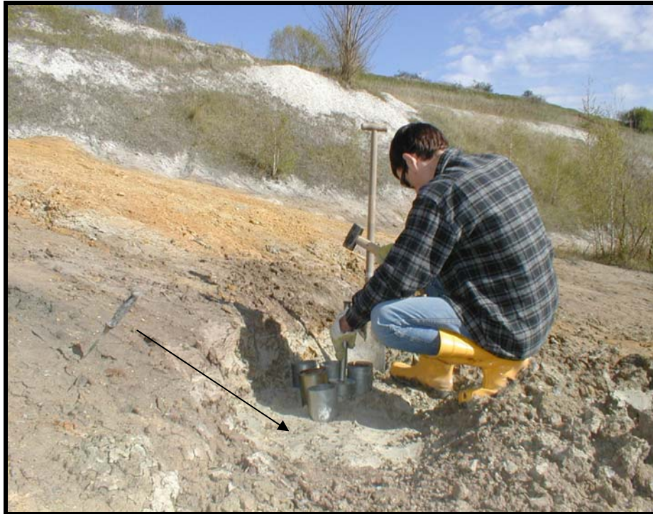
Fig. (2.6) Weathered soil of Muschelkalk Formation is collected from old quarry between Zappendorf and Koellme villages (NW of Halle city).
