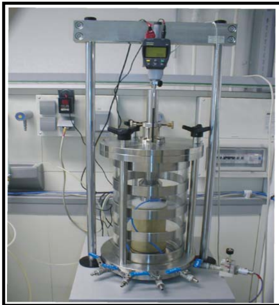
Fig. (2.10) Computerized triaxial cell to measure the unconfined compressive strength ( \sigma_3 = \text{zero} ).
