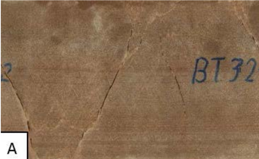
Figure 1: Unrolled combined photographs of a cylindrical sandstone sample after a multi-stage triaxial test with \hat{\sigma}'_3 > \hat{c}' except at the onset and near the endplates (LEMPP et al. 2020)
