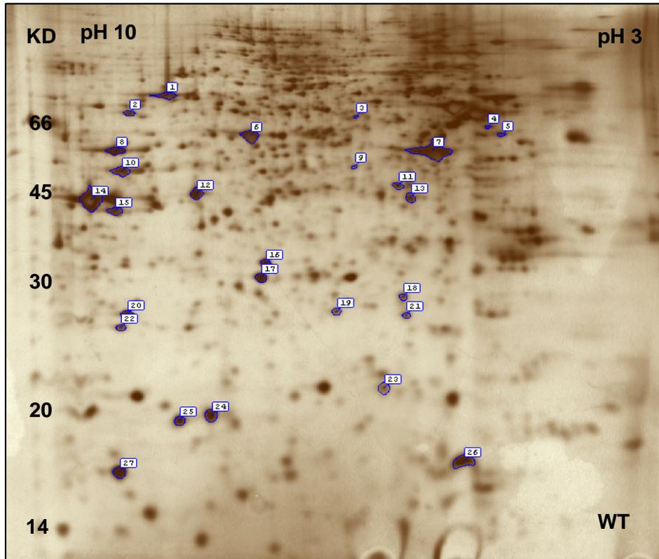
Figure 22: Reference gel with the reference spots of wild type FTC-133 cells after silver staining.
