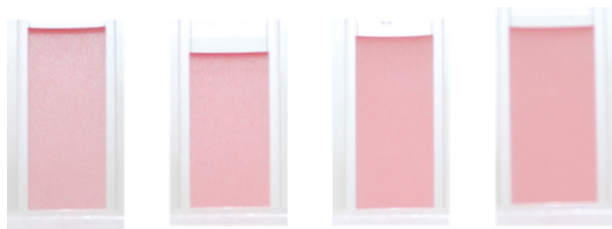
Figure 3. Initial state of the emulsion as obtained immediately after homogenization at 6000, 8000, 10 000, and 12 000 rpm (from left to right) during 30 s.
