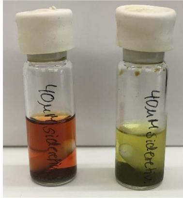
**Fig. 3. Sideretin stock solutions before (left) and immediately after (right) reduction with hydrogen in the presence of palladium.**
