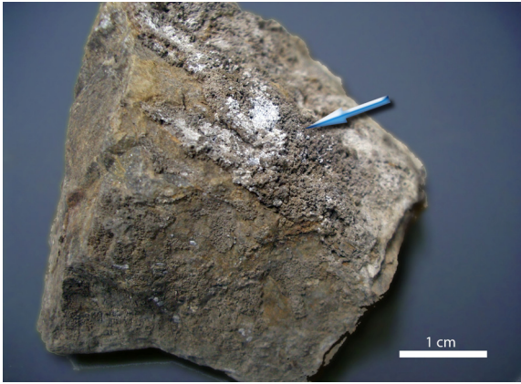
Fig. 69: Type-A non-sulphide ore on fracture-planes. The non-sulphide ore minerals occur exclusively on the fractures planes (arrow). The adjacent massive dolomite is not mineralised. Sample No. IK02114.
