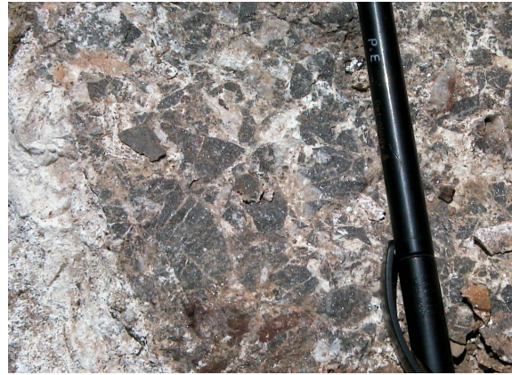
Fig. 70: Matrix supported breccia, which is characterised by angular fragments with a sharp contact to the fine-grained non-sulphide cement. The fragments match along their opposed sides, indicating only modest disturbance.
