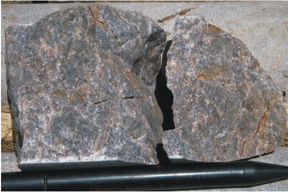
Fig. 75: Dolomite of DDH64 at 12 m. The dolomite is gray to dark grey coloured. Fractures are coated with Fe-hydroxides.
