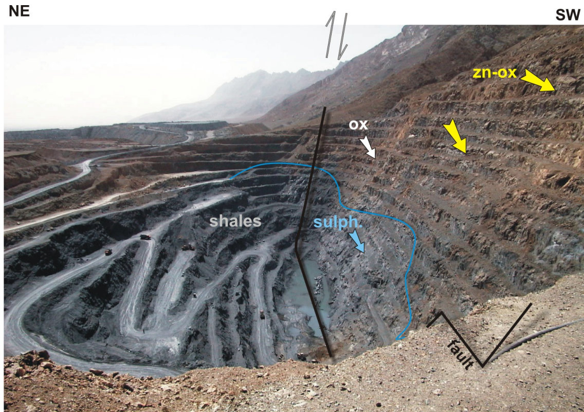
Fig. 59: View of the Goushfil pit at the Iran-Kuh district. Cretaceous dolomite in the south and Jurassic shales in the north are separated by a W-E trending fault. The vertical zonation (marked by the blue line) separates a non-oxide zone (dark grey colours) in the lower parts of the deposit and an oxide-zone (brown colours) in the upper parts. The sulphide ore is mainly hosted in the dolomite (blue arrow). The non-sulphide ore occurs within the oxide zone as secondary mineralisation predominately in the vicinity of faults and fractures (yellow arrows).
