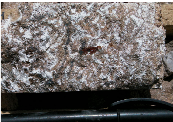
Fig. 78: DDH64 at 111 m. The dolomite is brownish-reddish coloured. The brownish dolomite clasts are (if visible) and remnants of them are highly altered and show diffuse edges due to replacement by smithsonite and hydrozincite (the dark red coloured area is caused by Zinc Zap, an indicator for non-sulph. zinc minerals).
