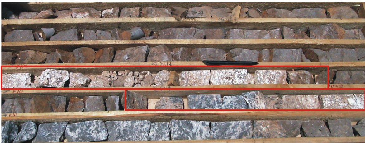
Fig. 77: Typical drill core sequence of borehole DDH64 with a zone of high-grade non-sulphide ore at 110 m (red marked). The non-sulphide ore consists mainly of cm-sized dolomite fragments that show a replacement by mainly smithsonite and hydrozincite, which also build the matrix of this breccia.
