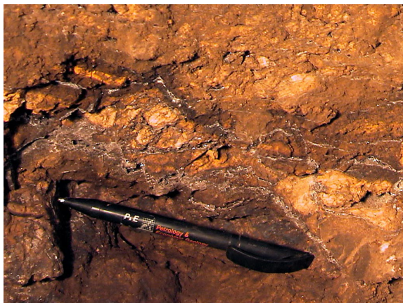
Fig. 14: Red zinc ore from MOB, adit no. 2. The reddish-brown colour is due to the high Fe-concentration of this ore type. Common minerals are goethite, hematite, hemimorphite, hydrozincite and traces of smithsonite.
