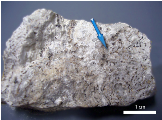
Fig. 69: Type-A non-sulphide ore on fracture-planes. The non-sulphide ore minerals occur exclusively on the fractures planes (arrow). The adjacent massive dolomite is not mineralised. Sample No. IK02114.
