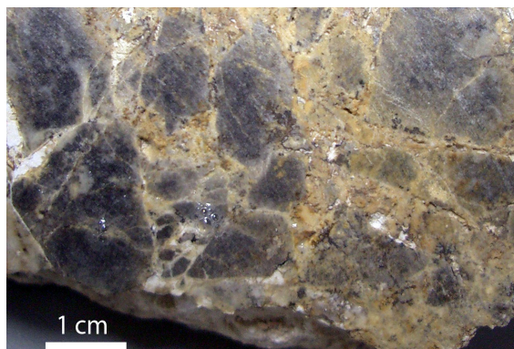
Fig. 68: Angular fragments of a breccia, cemented by non-sulphide Zn-(Pb-) minerals (hydrozincite, smithsonite, cerussite and subordinate amounts of iron hydroxides).
