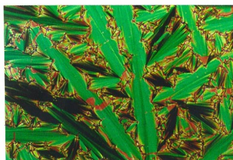
Figure 3-13 Optical photomicrograph (crossed polarizers) of the fan texture of 17/6 as obtained by cooling from the liquid state at 194^\circ\text{C} .
