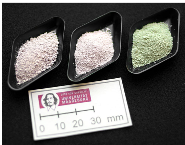
FIGURE 2 (\text{AlCr})_2\text{O}_3 powders obtained after calcination at 1000°C with 1.25 mol% \text{Cr}^{3+} (left), 2.5 mol% \text{Cr}^{3+} (middle) and 5.0 mol% \text{Cr}^{3+} (right)
