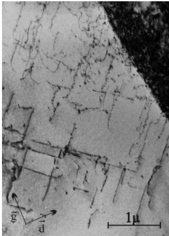
6.2.1. Microstructure of \text{ZrO}_2\text{-10mol\%Y}_2\text{O}_3 deformed along \langle 100 \rangle at 700°C till \epsilon = 1.3\% , shown with the [020] \vec{g} -vector at [001] pole
