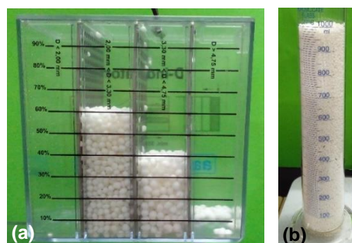
Figure 1: Measurement of (a) the particle size distribution and (b) the bulk density
