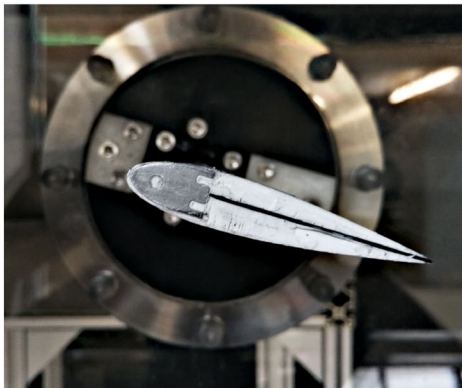
Fig. 2 (Left) section of a bioinspired flexible hydrofoil, displaying the solid leading edge on the left, a flexible carbon-fiber composite skeleton, surrounded by a white silicone embodiment. (Right) Hyperflexible structures adapt to the flow and can inhibit or milden dynamic
